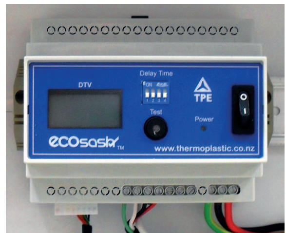
The EcoSash® Controller, common to both new fume cupboard installations and to retrofits.
