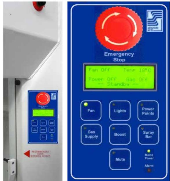
The Fixed Volume (CAV) Controller comes with a vertically oriented, touch-type control panel that can be mounted on either the left or right column of a fume cupboard. This example shows the control panel mounted on an EcoAir® fume cupboard.
