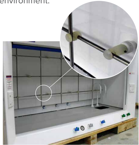
Factory view of fume cupboard with scaffolding system fitted.
