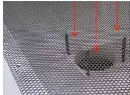
Perforated work surface/inlet grill (Stainless steel option shown).
